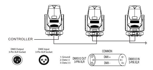
For installations where the DMX cable has to run a long distance or is in an electrically noisy environments as in a disco, it is recommended to use a DMX terminator. This helps in preventing corruption of the digital control singal by electrical noisy. The DMX terminator is simply an XLR plug with a 120 resistor connected between pins 2 and 3, which is then plugged into the output XLR Socket of the last fixture in the chain. Please see illustrations
