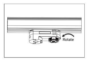
Step 2 When power knob at the "OFF" position, rotate the hand grip at 90 degree.
